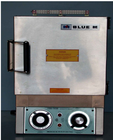
Figure 23 - Blue M Stabil Therm Gravity Oven used for drying of treated chabazite
