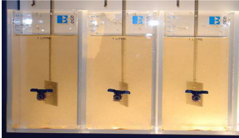
Figure 27 - Kinetic studies jar tester configuration
