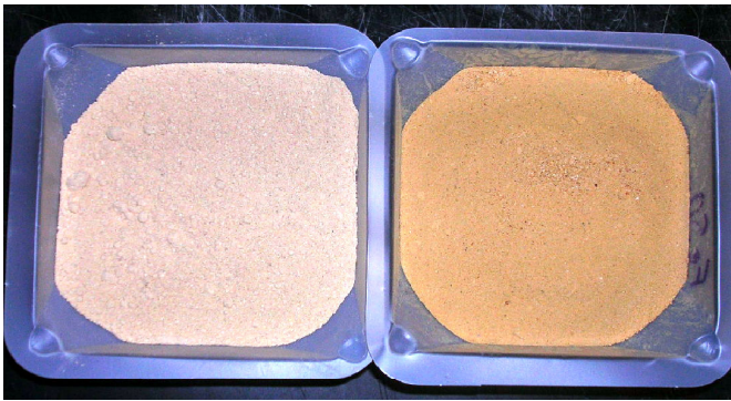
Figure 26 - Chabazite before and after iron (II) sulfate modification
