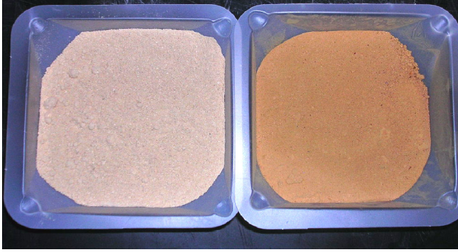
Figure 25 - Chabazite before and after iron (II) chloride modification
