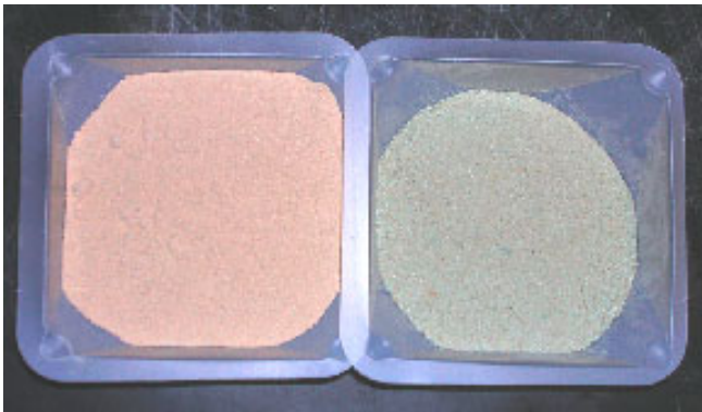
Figure 24 - Chabazite before and after copper (I) chloride modification
