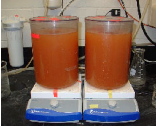
Figure 20 - Batch reactors for pretreatment of chabazite using various reagents
